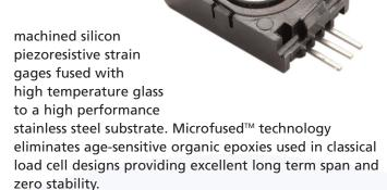
Operating at exceedingly low strains, Microfused<sup>™</sup> technology provides gage factors greater than 100, an essentially unlimited cycle life expectancy, superior resolution, exceedingly high over-range margins without the need for stops and a ratiometric span of 3V. Microfused<sup>™</sup> sensors are used in a variety of applications including bathroom scales, paint sprayers and safety-critical automotive brake sensors.
